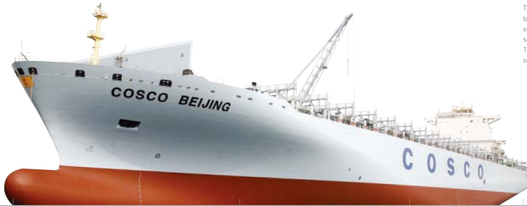
Cosco Beijing Containership • Sister ship to Cosco Guangzhou, the industry's first 9,500 TEU-class vessel • Delivered in June 2006, the second of a five-ship order
