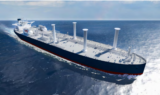
Hi-Rotor(New concept eco-friendly sail)
