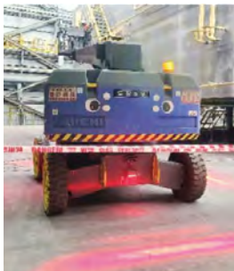
cherry picker operation performed after setting up warning lights and barricades (improvement)
