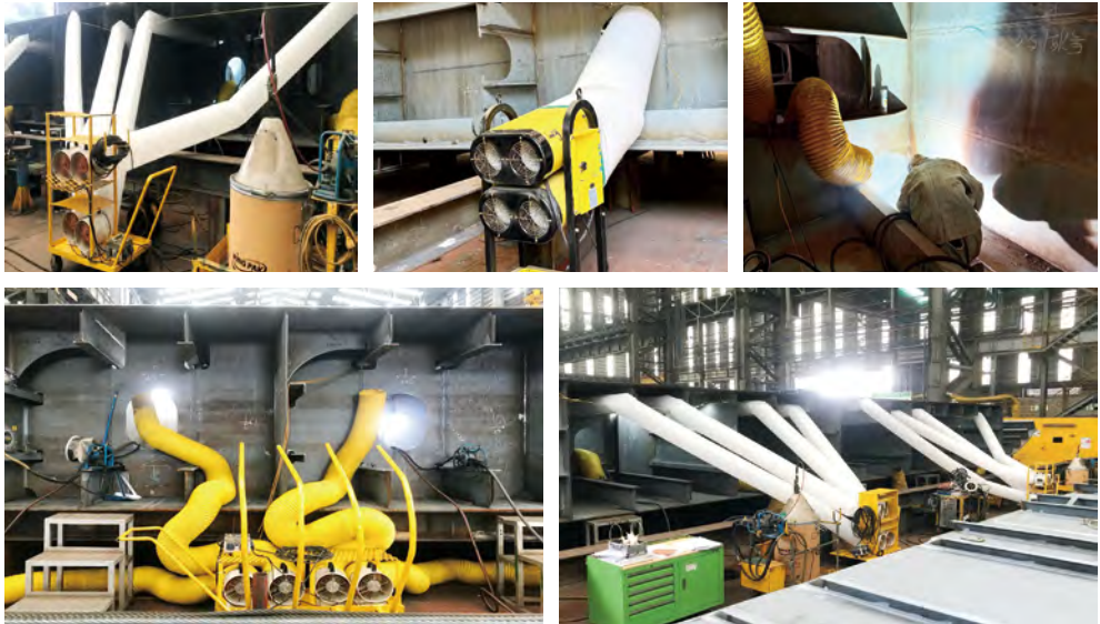
Ventilation using exhaust and intake systems with automated noise reduction equipment
