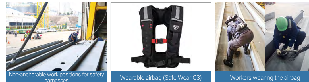
A wearable airbag to reduce fall injury rates for workers working on block tops
